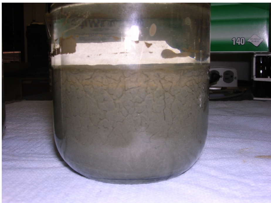
Figure 32: Side View of Microcosm with Evidence of Burrowing into the New Bedford Harbor Marine Sediment Diluted with Brown's Lake freshwater Sediment.
