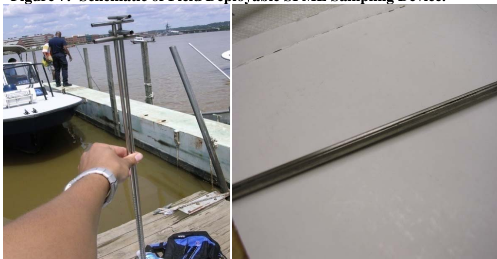
Figure 8: Picture of Field Deployable SPME Sampling Device.
