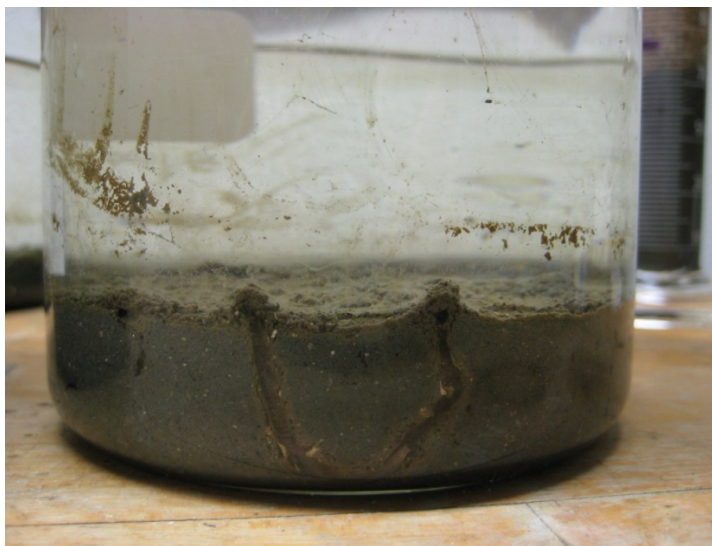
Figure 24: Hunter's Point Sediment Microcosm – Side View with Evidence of Neanthes Burrowing.
